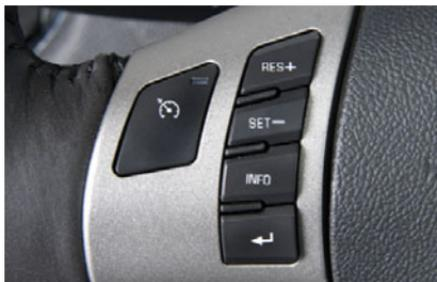
The following cruise control buttons are located on the steering wheel:
