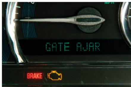
Your vehicle's Driver Information Center (DIC) provides vehicle information, vehicle feature personalization and vehicle warning messages. The DIC messages will be shown on your instrument panel cluster display. To operate the DIC, the ignition switch must be in the Run position.
