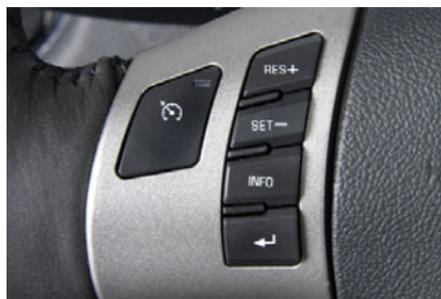
The DIC is controlled through the following two buttons located on the left side of the steering wheel:
