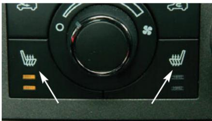
There is a heated seat control button located on the climate control panel for each front seat.
