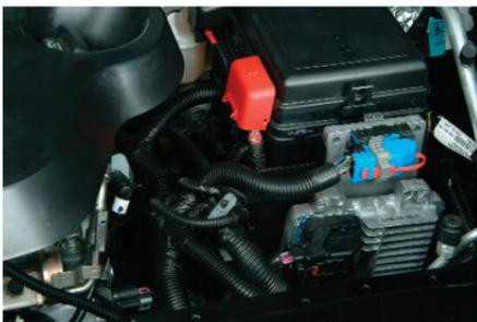
The battery is located in the spare tire well, under the floor in the rear cargo area. Should it be necessary to jump-start your vehicle, use the remote positive terminal (located under the red cap) and the remote negative ground terminal (marked GND) in the engine compartment on the driver's side strut tower.
