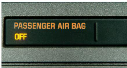
Your vehicle is equipped with a Passenger Sensing System located in the front passenger seat for the front passenger frontal airbag, and a passenger airbag status indicator located on the center of the instrument panel.
